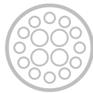
SG16 Cavity Configuration 12 x Ø 1.6mm Contacts 4 x Ø 3.5mm Contacts
